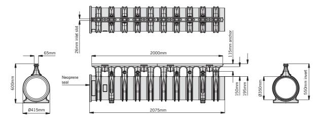
ACO Qmax® 350 with ACO Q-Flow ductile iron edge rail
