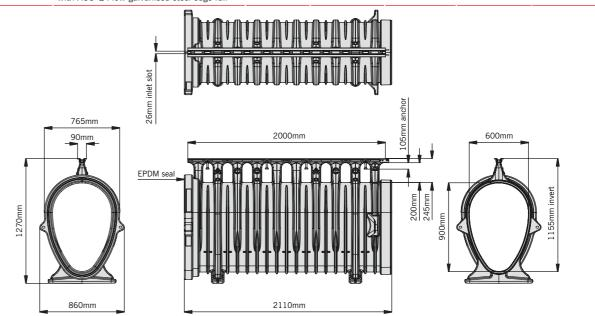
ACO Qmax® 900 with ACO Q-Flow galvanised steel edge rail
