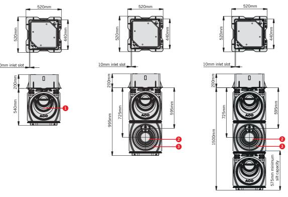
ACO Qmax® 150, 225 and 350 access chamber with D 400 ACO Q-Slot
