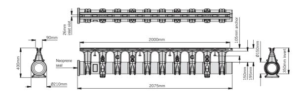
ACO Qmax® 150 with ACO Q-Flow galanised steel edge rail
