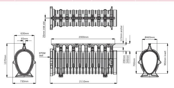
ACO Qmax® 700 with ACO Q-Flow ductile iron edge rail
