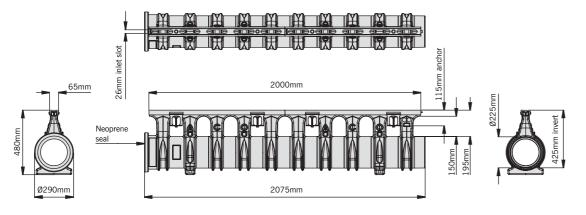
ACO Qmax® 225 with ACO Q-Flow ductile iron edge rail
