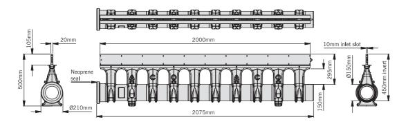
ACO Qmax® 150 with ACO Q-Slot galvanised steel edge rail
