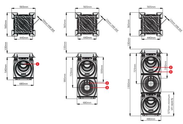
Image shows ACO Qmax® 150, 225 and 350 access available in Load Class F 900.
