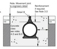
For Load Class F 900 it may be necessary to reinforce over, under and to the sides of the unit (as indicated). Engineering advice should be sought.
